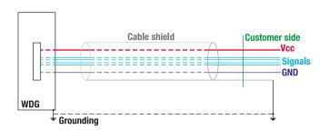
L2/L3, T3: Cable shield connected to encoder housing. Encoder housing not earthed separately.
