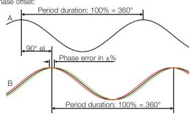
El. phase offset:  $90^{\circ} \pm \text{max.}$  phase error 7,5% of a period duration
